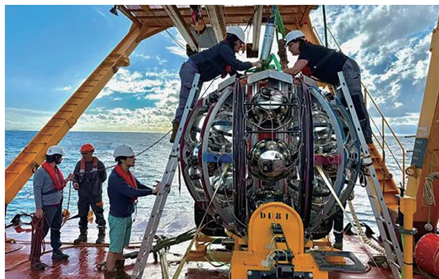
Engineers prepare to install a detector into the underwater KM3NeT network. (Image credit: Paschal Coyle CNRS)
