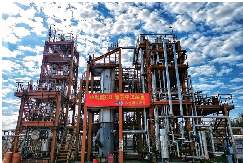
A 1,000 ton/year CO 2 hydrogenation to gasoline pilot plant.
