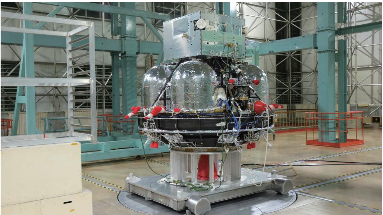
Fig. 5. Magnetic testing of the SMILE flight model.
